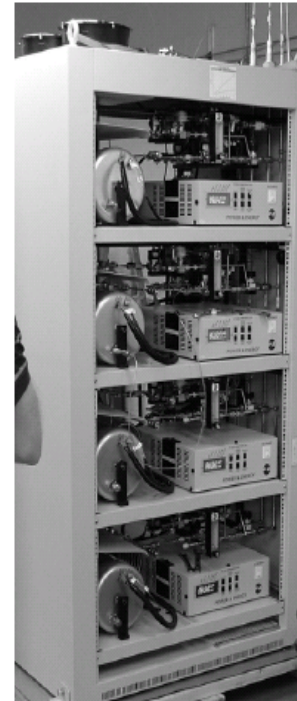
High Capacity 1300 slpm Modular H 2 Purifier System
