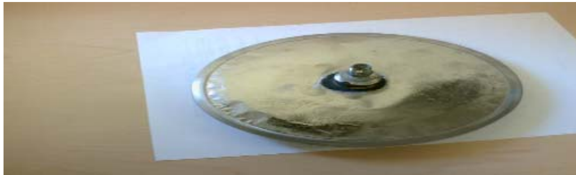
Disc and doughnut design of a hydrogen separation system
