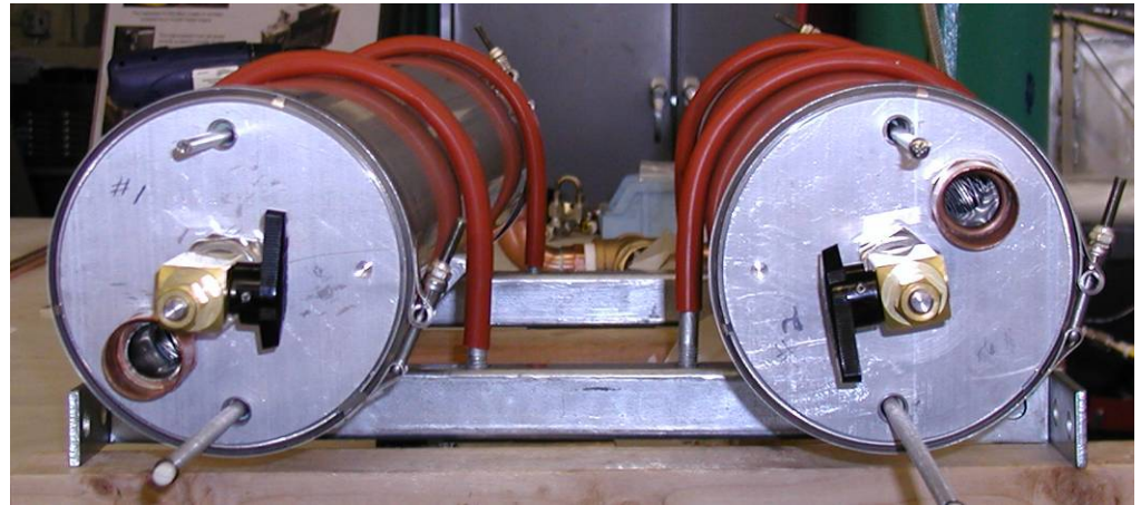
Each heat exchanger contains 3 stages to compress hydrogen from 0.5 bara to 100 bara
