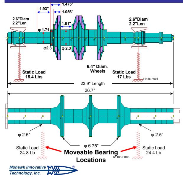
60,000 rpm Compressor Concept Design
