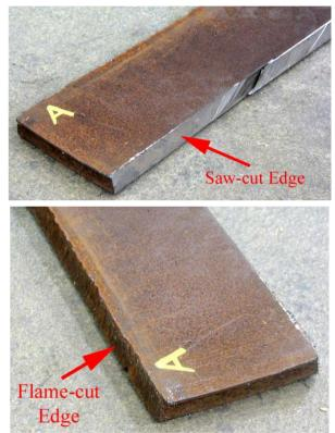
A strip of material measuring approximately 6' long and 4" wide was supplied from a 30-36" diameter X100 pipe by NIST-Boulder
