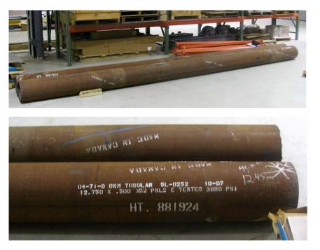
Approximately 40' of 12.75" OD, 0.5" thick, electric resistance welded (ERW) X52 pipeline was procured from Oregon Steel Mill's Tubular Camrose facility in Alberta, Canada
