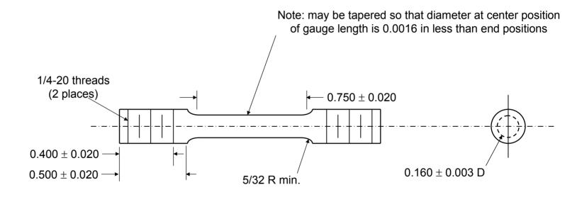
All dimensions are in inches. Maximum RMS surface roughness = 8 microinches
