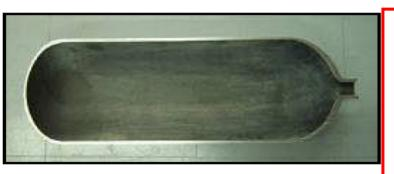
Performance of liner in hydrogen is currently unknown, but high strength suggests embrittlement concerns. For scale-up, a more suitable alloy should be selected and incorporated in overall COPV design.
