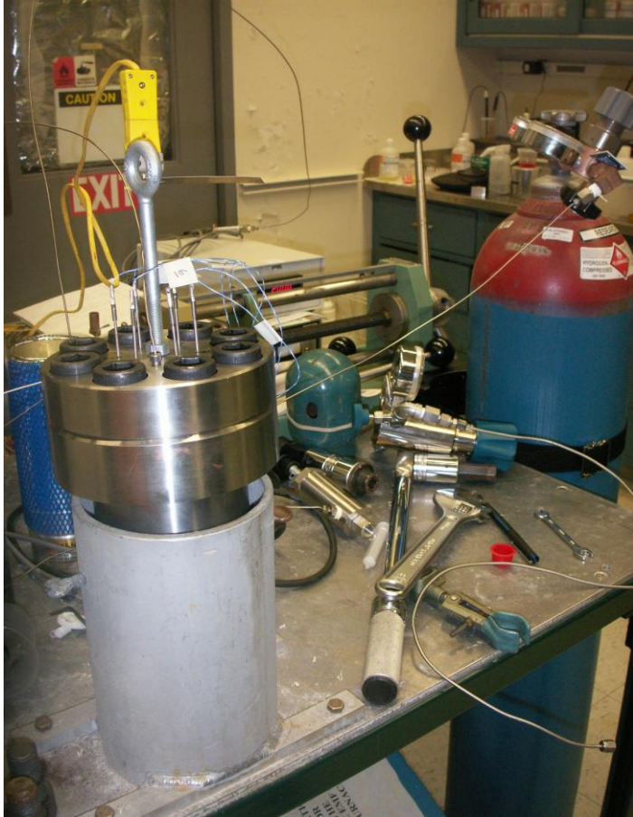
Pressure vessel and instrumentation for HE test
