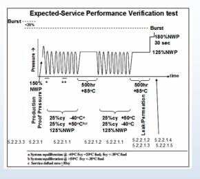
Post test burst strength determination
