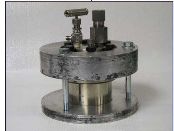
HPHE Milling Reactor 33
