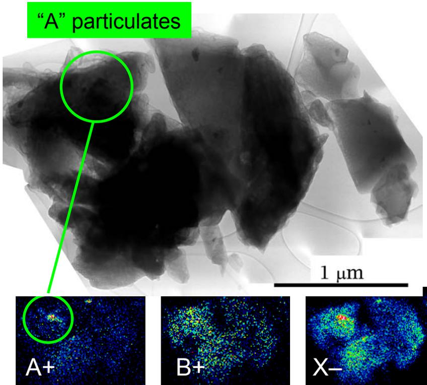
$\text{Ca}(\text{BH}_4)_2$  + 3 wt % "A" + 3 wt % "B", after 2<sup>nd</sup> cycle, dehydrided state – Ru region ~ 100 nm
