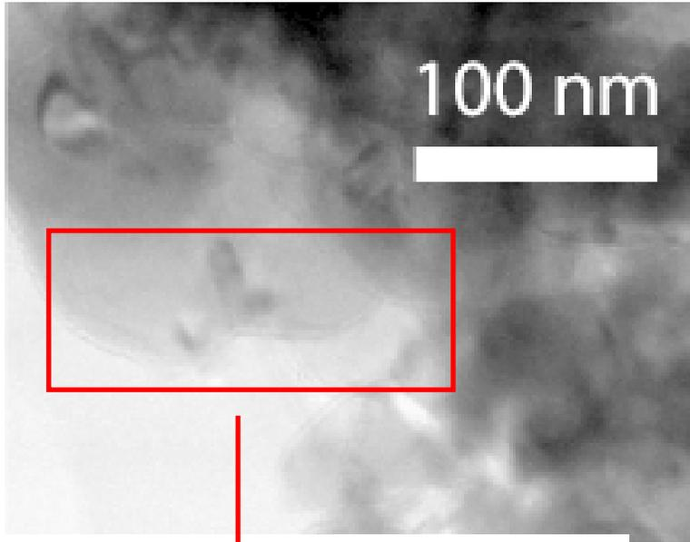
No enhancement of local Ti conc. at edge of Al particle.
