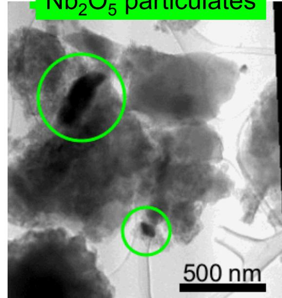
$\text{MgH}_2 + \text{MgB}_2 + 2\text{B} + 0.02\text{Nb}_2\text{O}_5$ , bright-field, after 1x hydrogen cycle.
