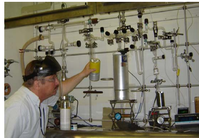
Glass vacuum line, teflon stopcocks, viton o-rings
