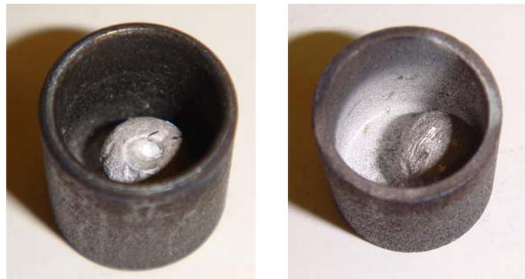
Image at left shows attempt to melt Mg in carbon crucible and shows no evidence of wetting. Original ingot morphology was cylindrical and turned spheroidal with poor contact angle. Image at right shows similar attempt when Ni film of several hundred Å is deposited into crucible before melt attempt. Some Mg coating of surface evident, presumably from Mg vapor phase.
