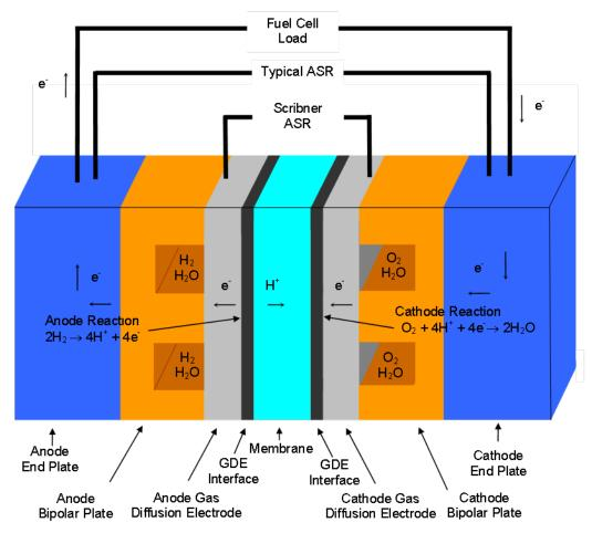
Component Resistance Plus Resistance at each interface <sup>39</sup>
