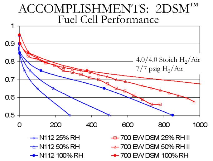
25% RH data much worse than predicted based on DSM<sup>™</sup> conductivity and high-frequency
