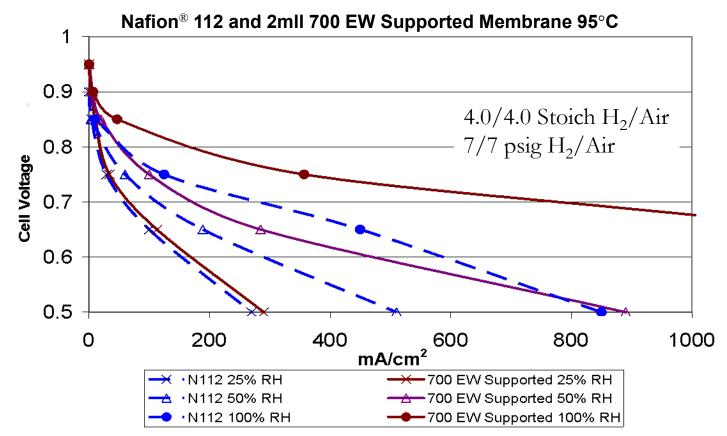
25% RH data much worse than predicted based on DSM<sup>TM</sup> conductivity and high-frequency resistance: Work to do on the catalyst layer
