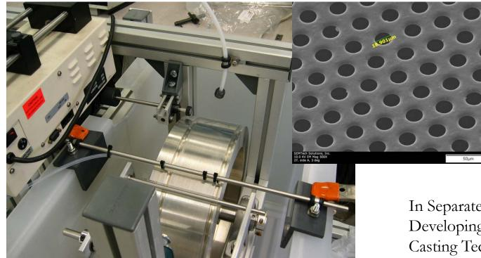
Automatic solution dispensing Automatic speed control Manual support collection Solution recycling can be implemented In Separate DOE Project Developing Low-Cost Casting Technique (**DE-FG02-05ER84322**) PI: Han Liu
