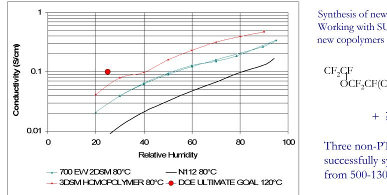
Synthesis of new PFSA Monomers Working with SUNY-ESF to make new copolymers and homopolymer
