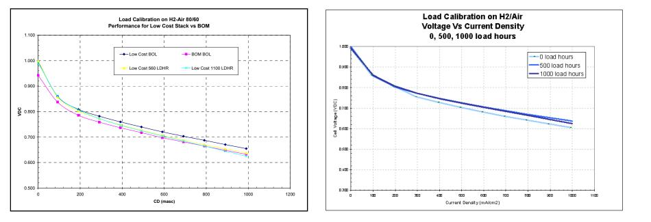
Low cost cell stack demonstrated performance equivalence with baseline design. No degradation observed over initial 1,000 hours of endurance testing.
