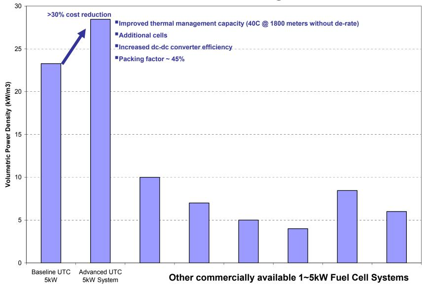
(Configured as standalone stationary power system: includes thermal mgt, power conditioning, startup battery)
