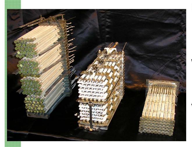
Number of tubes for 1.25 kW reduced from 126 to 72 to 45
