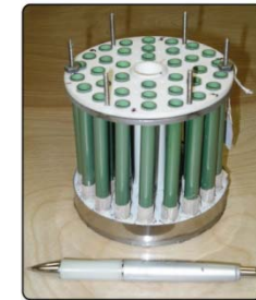
Example configuration of 250-W tube bundle
