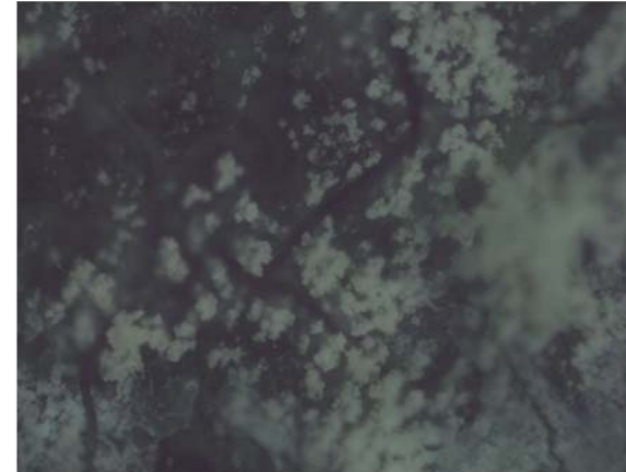
Optical image of carbon foam deposited with nickel oxyhydroxide (200X).
