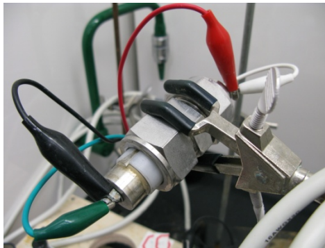
Swagelok cell connected to a potentiostat for cycling
