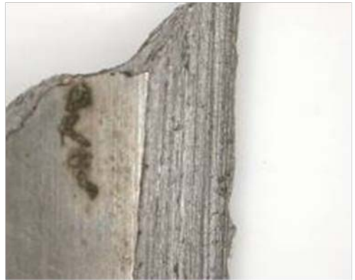
Cross section of failed Ta-10W 2" dia vessel
