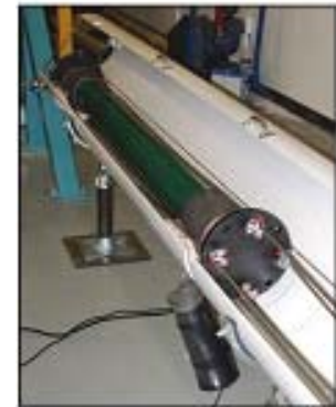
Leakage Measurement at Oak Ridge
