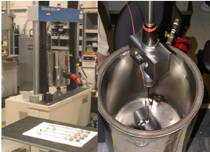
Tension test at cryogenic conditions
