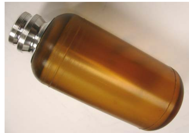
February 2009: Early liner production tooling dialed in, first pressure tests with a low-P boss
