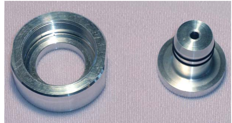
February 2009: Early liner production tooling dialed in, first pressure tests with a low-P boss
