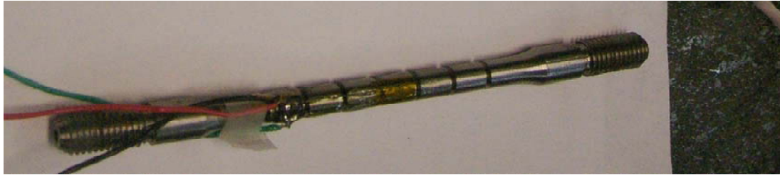
Miniature notch tensile specimen (3mm dia.) with notches to sample different microstructures in weld, HAZ and base metal for comparative evaluation
