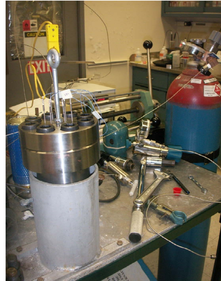
Pressure vessel and instrumentation capable of multiple tests at a time
