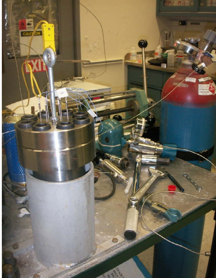
Pressure vessel and instrumentation for HE test
