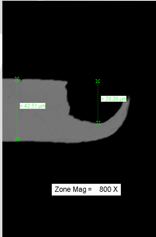
Cross-section of membrane failure point
