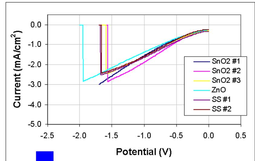
Photocurrent at zero bias is much smaller than in the 3-electrode set up, suggesting existence of limiting factors such as, type of **electrolyte**, **counter electrode** and formation of **SiO<sub>x</sub>** on the surface.
