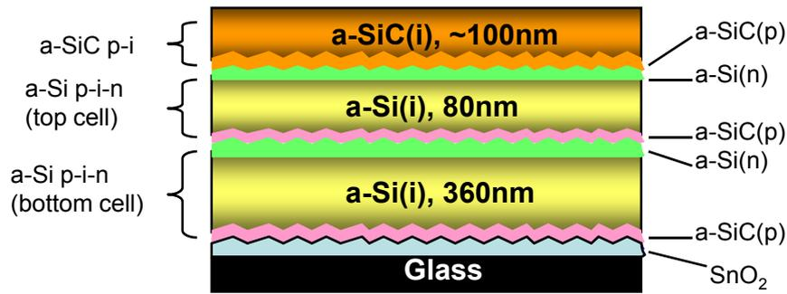
A-Si tandem solar cell --- major component in the hybrid PEC cell
