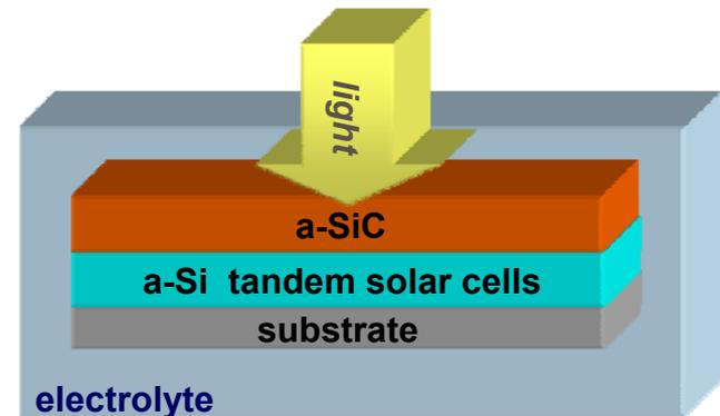
Schematic diagram of the PV/a-SiC hybrid device.
