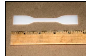
Liner test specimen
