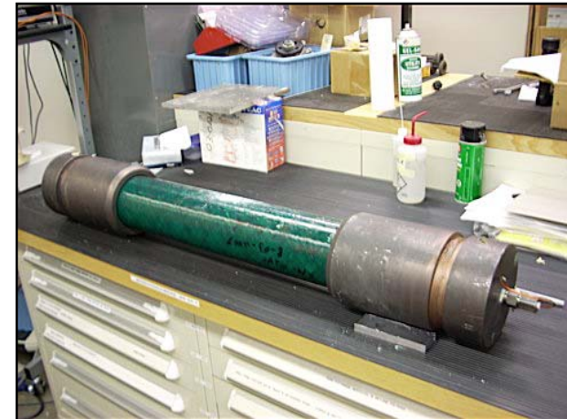
3-ft pipeline specimen being instrumented for blowdown testing
