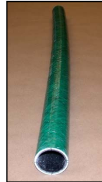
4-pt bending test specimen
