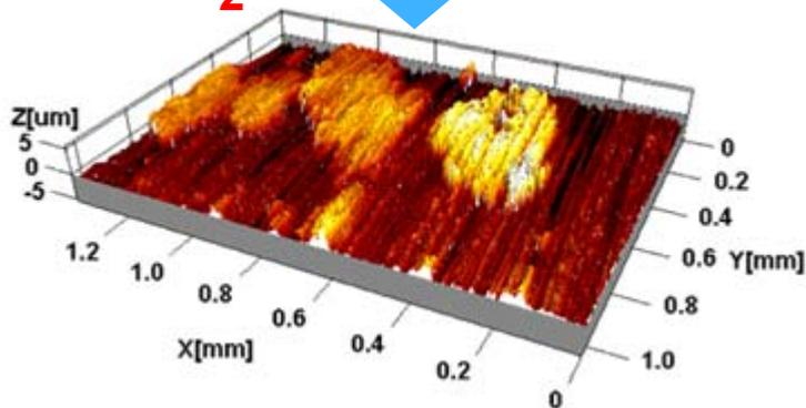
–Dark metallic galling marks on counterface after testing in air (oxide film)
