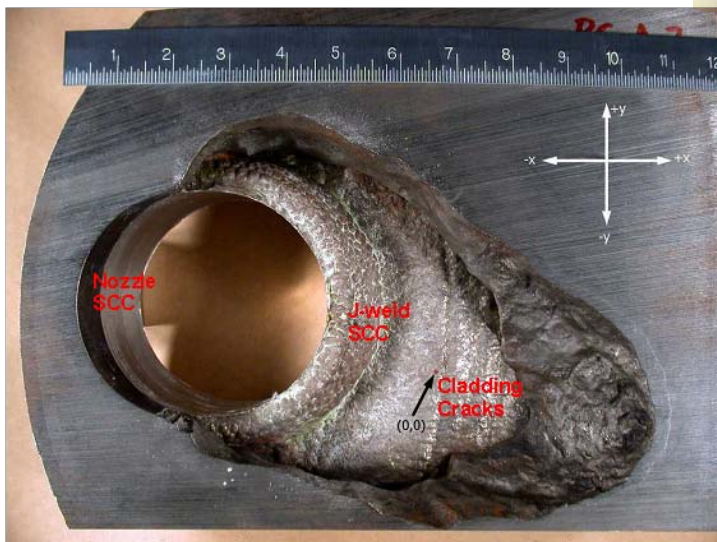
Example of materials degradation in hydrogen environment
