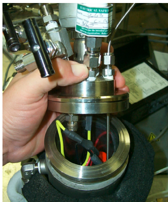
Metal-Insulator-Metal capacitor bank (left) and enclosure vessel with electrical leads (right) used in proof-of-concept experiments.
