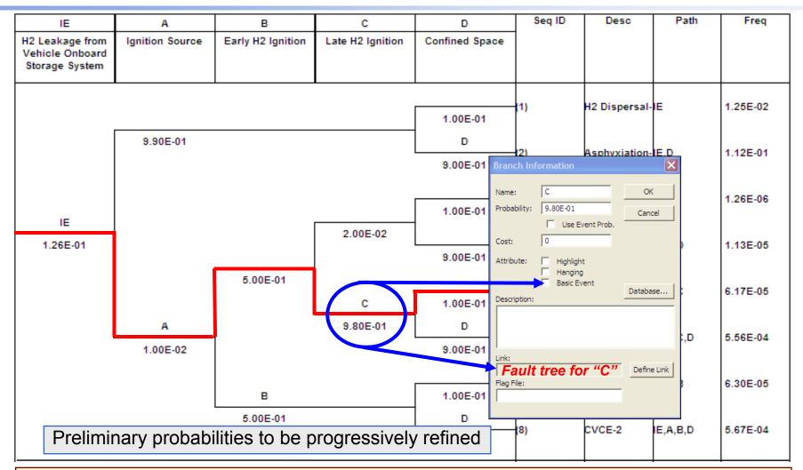
In CAFTA, a branch probability can be derived from a detailed Fault Tree or a Basic Event with a probability distribution to address uncertainties.
