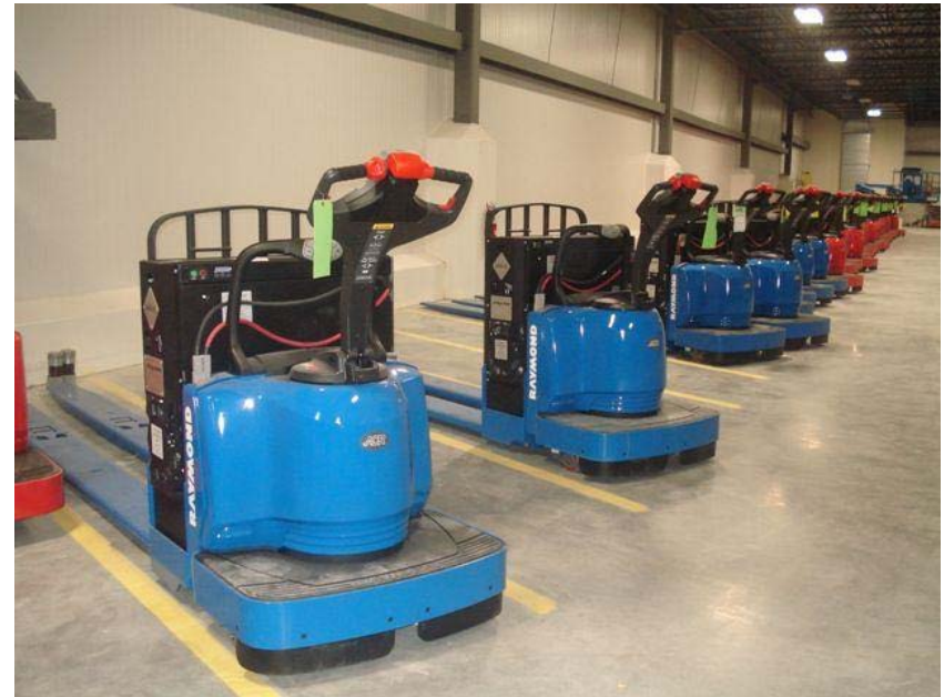
Fuel Cell Powered Lift Trucks (Sysco)
