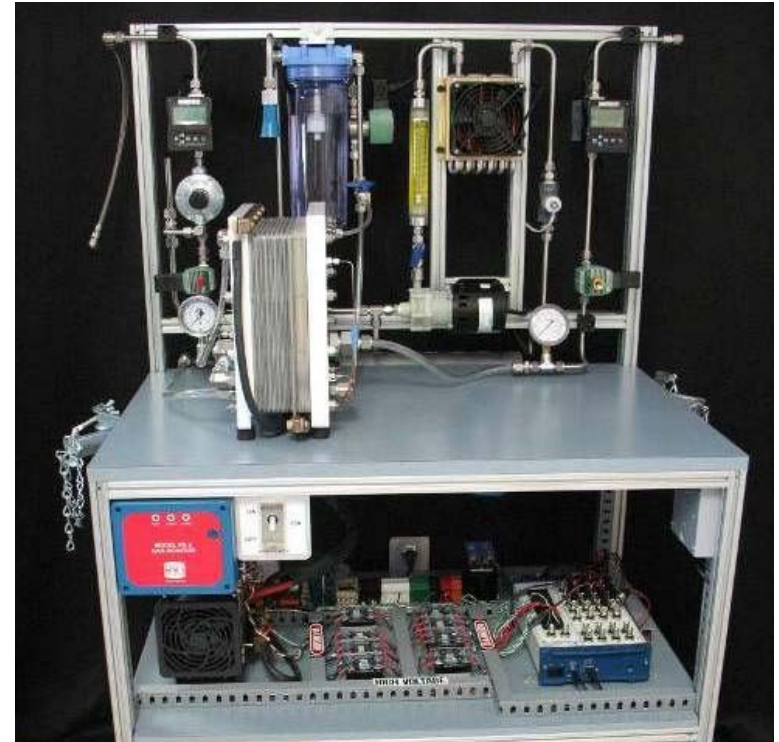
Hydrogen Fuel Cell Test Station
