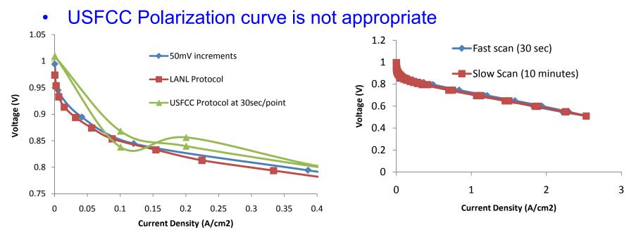
Cell Temp = 80°C. Anode and Cathode inlet RH = 100% (Not 50%). Anode and Cathode Outlet Back Pressure = 28.7psig (Los Alamos) = 40 psia  $H_2$  Flow : Minimum = 42 sccm and 1.2 stoich (50cm<sup>2</sup> cell) = stoich flow for 0.1A/cm<sup>2</sup> Air flow : Minimum = 166 sccm and 2.0 stoich (50 cm<sup>2</sup> cell) = stoich flow for 0.1A/cm<sup>2</sup> 2way scan: First range = 1V to 0.8V @ 20mV steps @ 30sec/step Second Range = 0.8V to 0.3V @ 50mV steps @ 30sec/step
