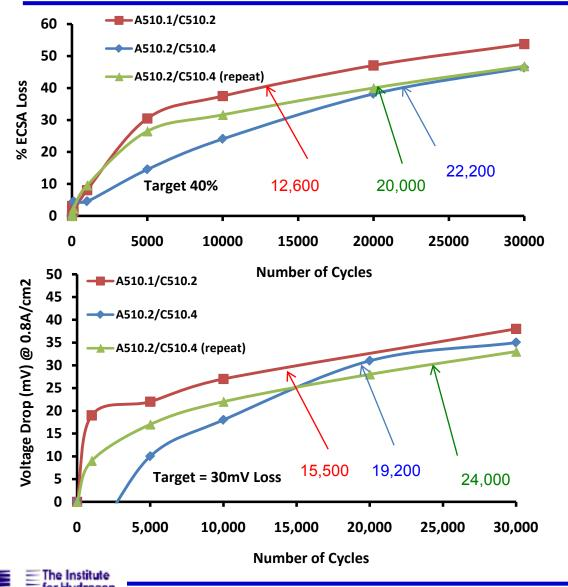
Performance loss accelerated at lower loadings
