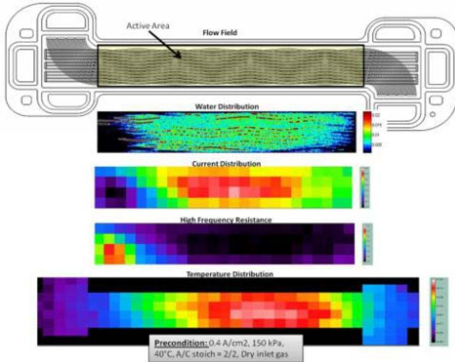
Local temperature, current density and HFR vary significantly for a given precondition
