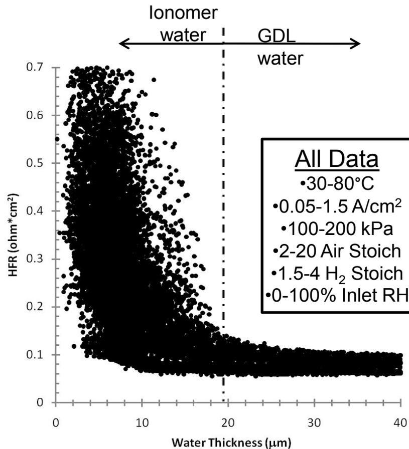
Direct correlation between HFR rise and water removal from GDL. Liquid water required in GDL to minimize HFR as transition is very sensitive.
