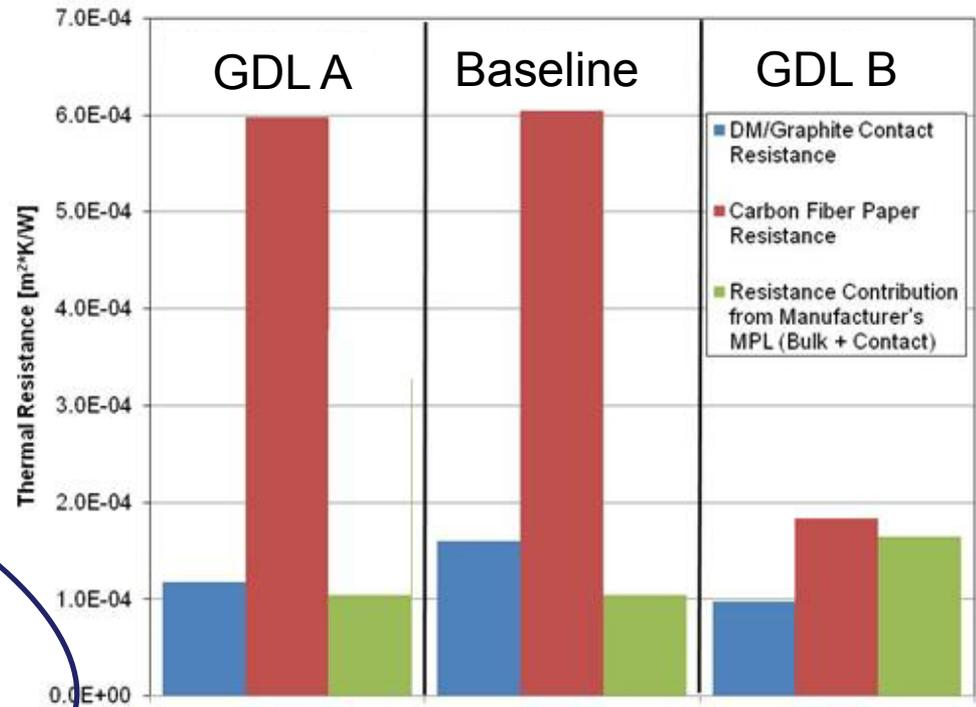
Higher thermal conductivity effectively lowers the saturation pressure near the MEA and more condensation in the bulk substrate results.
