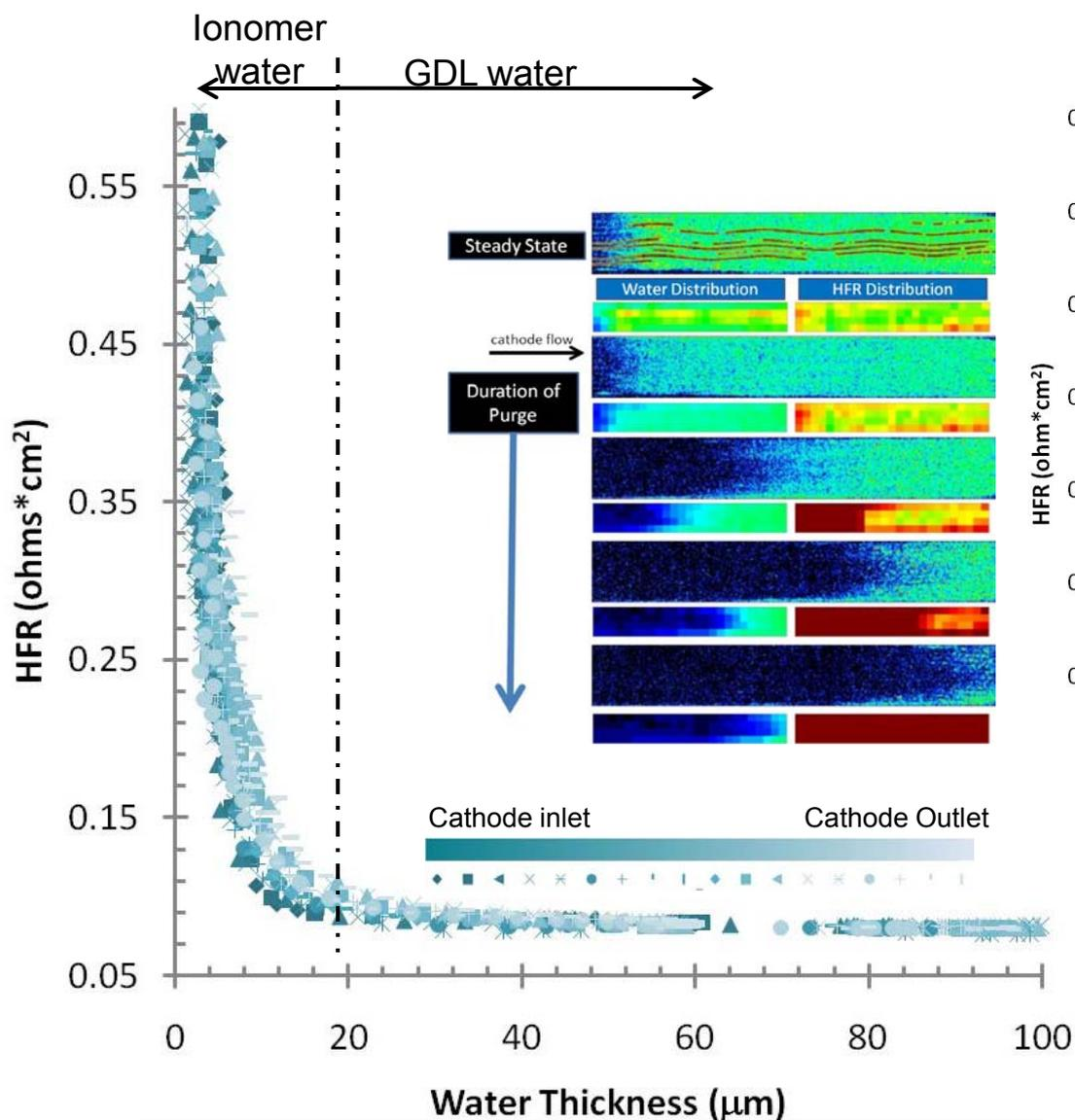
**Purge condition:** 100 kPa, 33°C, 1 SLPM N<sub>2</sub>, Dry inlet gas
