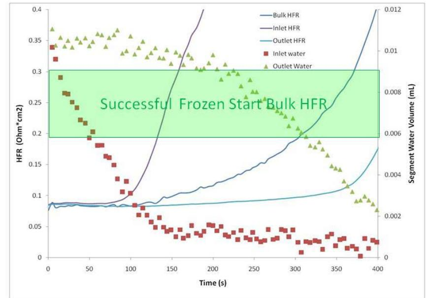
Once the saturation state for a precondition is understood, the relationship of local HFR increase with drying must be known to optimize purge conditions and materials for successful starts that have an even current distribution. Bulk HFR measurement is not sufficient.
