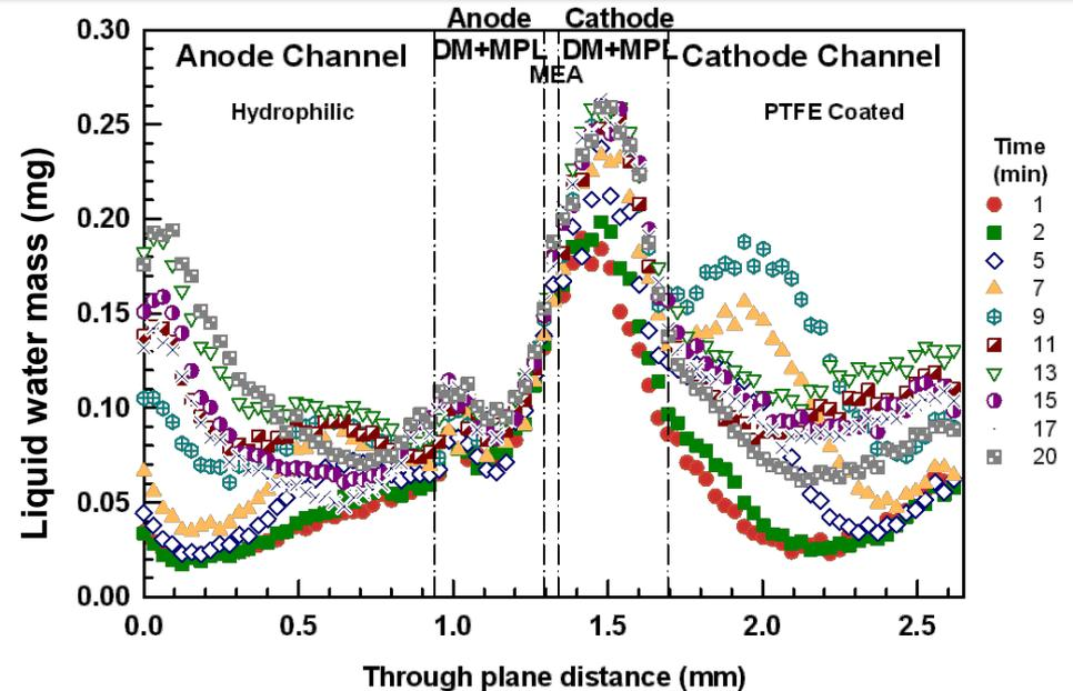
**Data show channel wall|DM interface plays a critical role in water drainage and overhead in DM and can be better engineered**
