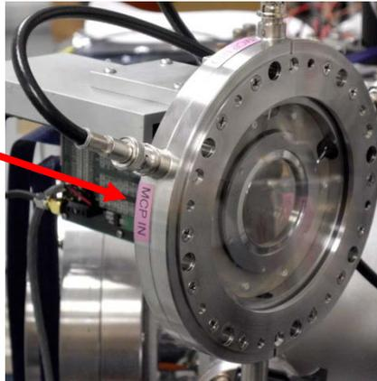
CCD/GadOx Detector System with <20  $\mu$ m spatial resolution will enable high resolution imaging of in-plane water content
