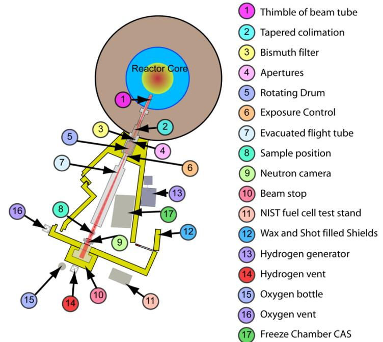
NIST Neutron Imaging Facility. Full facility capabilities provided in supplemental slides.
