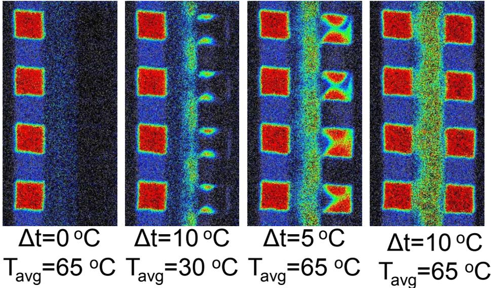
4 layer DM stack was bound by MPL on outside edges, with liquid initially on left side only and temperature gradient induced by coolant.
