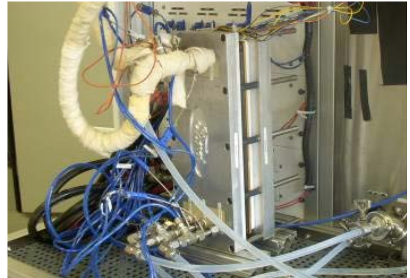
Ford short stack with metal bipolar plates
