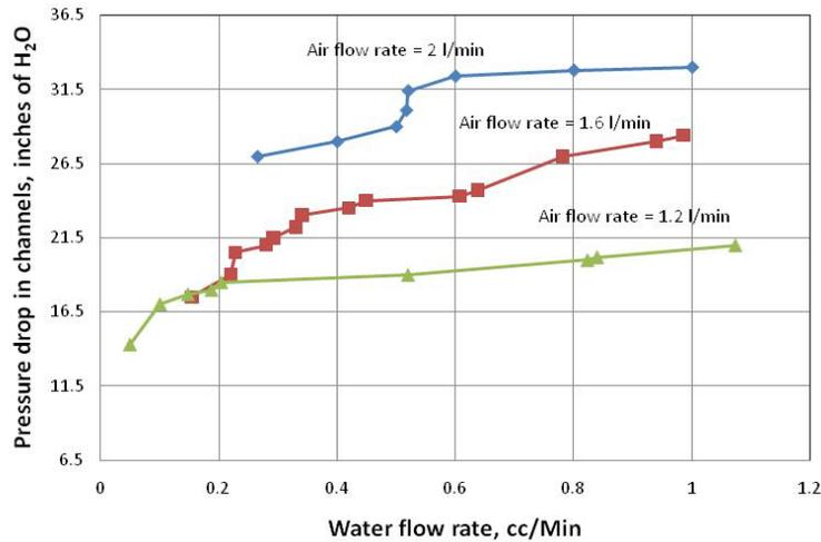
**Simultaneous film flow and slugs**
