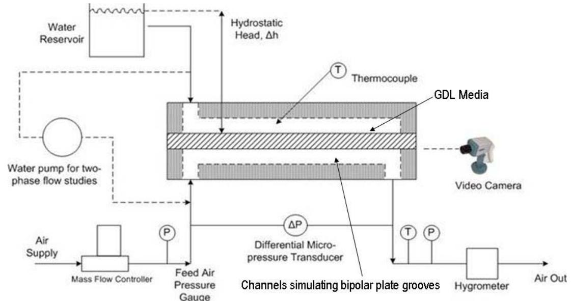
**Schematic of Water Transport Visualization Apparatus**
