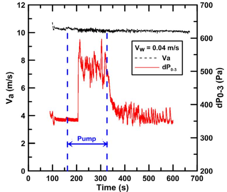
Typical differential pressure ( $dP_{0-3}$ ) signal in a two-phase flow channel measure between P0 and P3.
