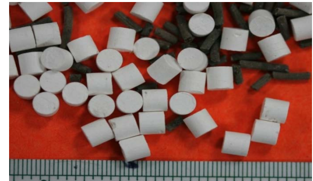
After slight discoloration with no conversion deterioration or breakage
