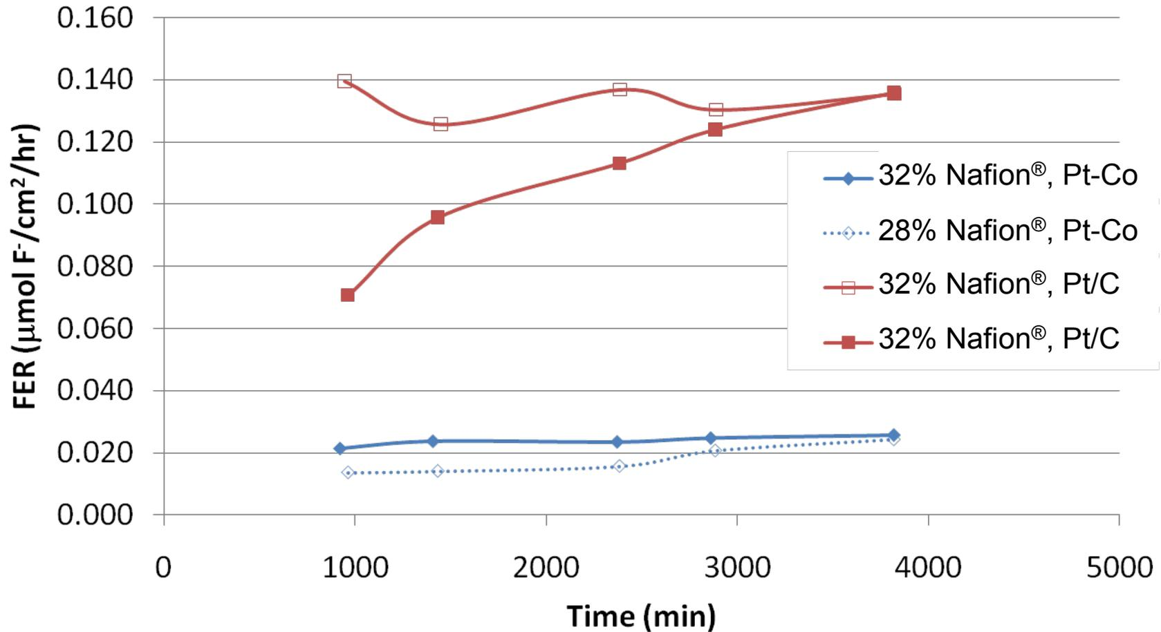
NRE 211 membranes with 1100EW Nafion<sup>®</sup> in electrode and Pt-Co or Pt/C catalyst.
