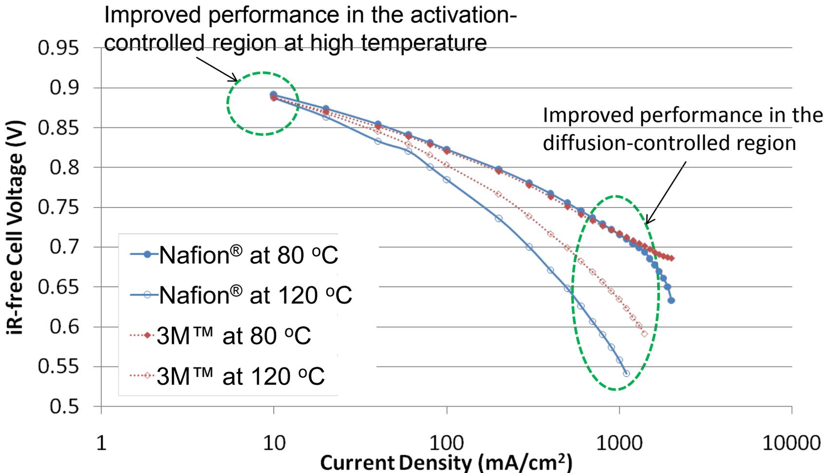
All tests were conducted with H<sub>2</sub>/air with 7psi backpressure
