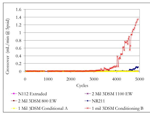
RH Cycling durability dependent on processing. 5000 Cycles demonstrated with 1-mil membrane.
