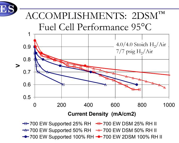
Reformulating the catalyst layer with same ionomer led to large improvement in performance
