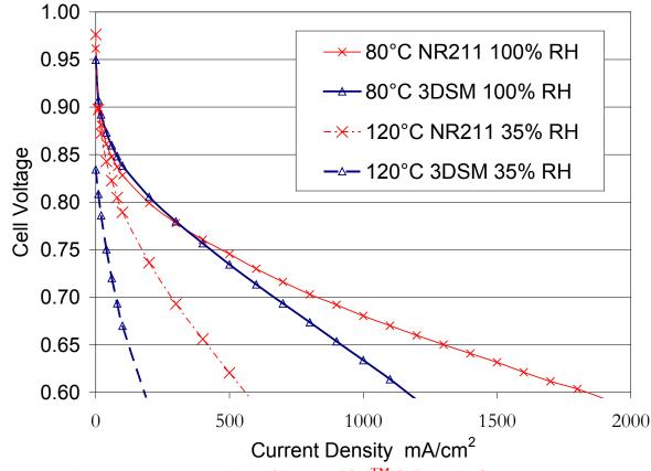
Poor performance is seen for the  $3DSM^{TM}MEA$ , however 1100 EW ionomer used in the catalyst layer.
