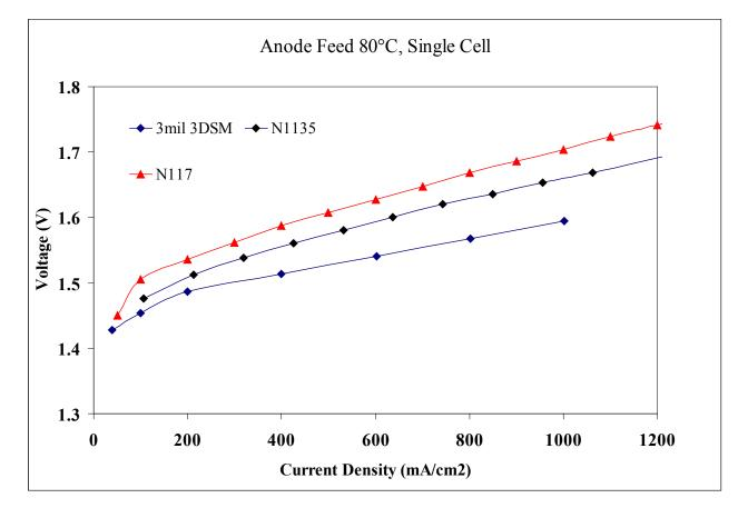
3DSM shows significant improvement to 1100 EW of comparable thickness
