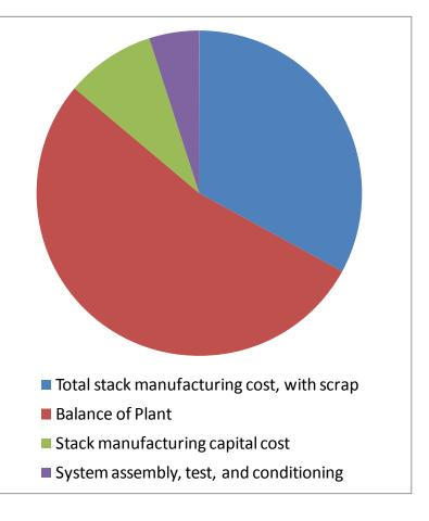
\* Stack cost based on high quantity manufacturing process in place. BoP cost based on purchase price for 2,000 units.
