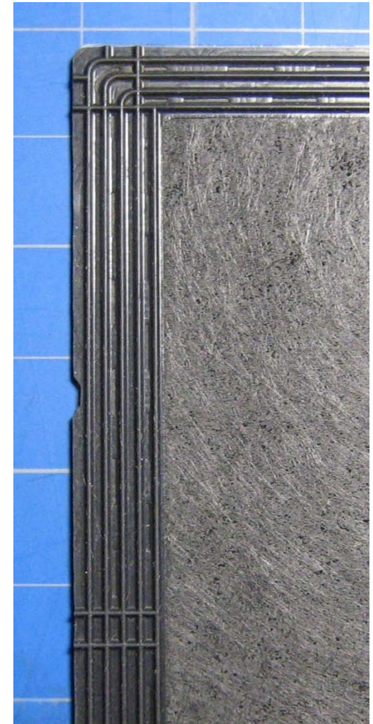
Full Size Prototype Made Using Hot-Runner LIM* tool
