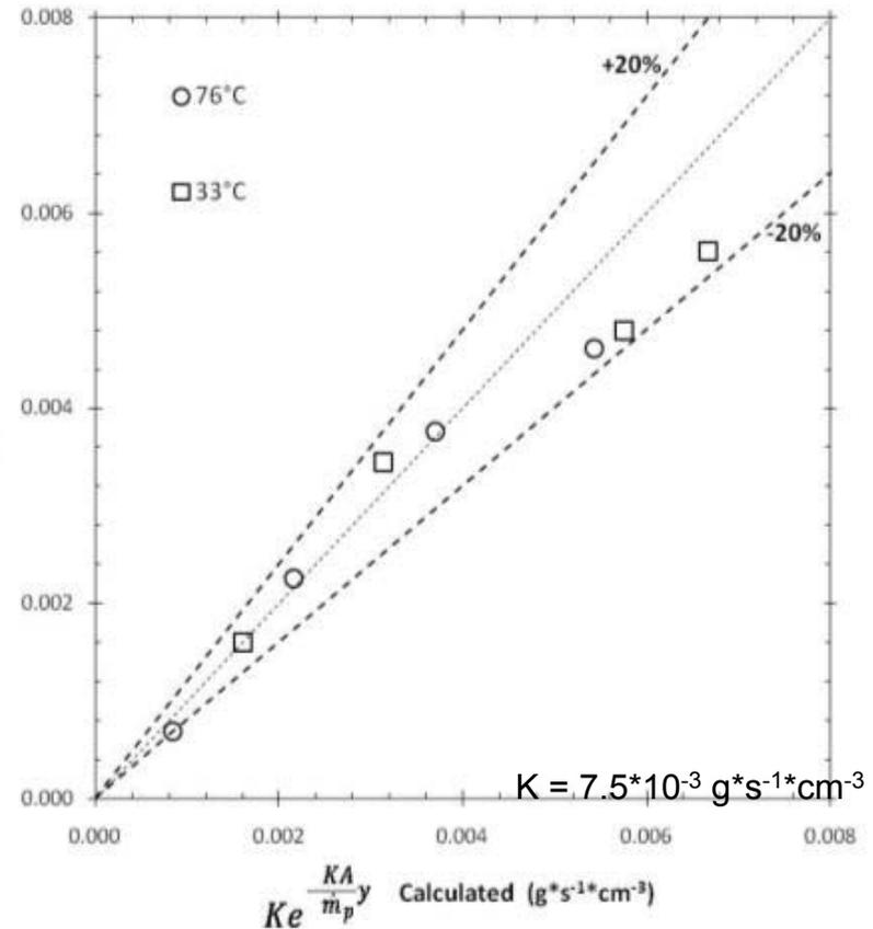
□ So... If the initial saturation state is known, purge drying is easily predicted.
