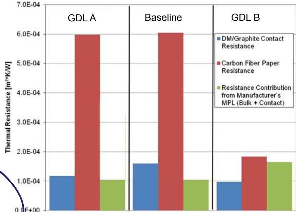
Higher thermal conductivity effectively lowers the saturation pressure near the MEA and more condensation in the bulk substrate results.
