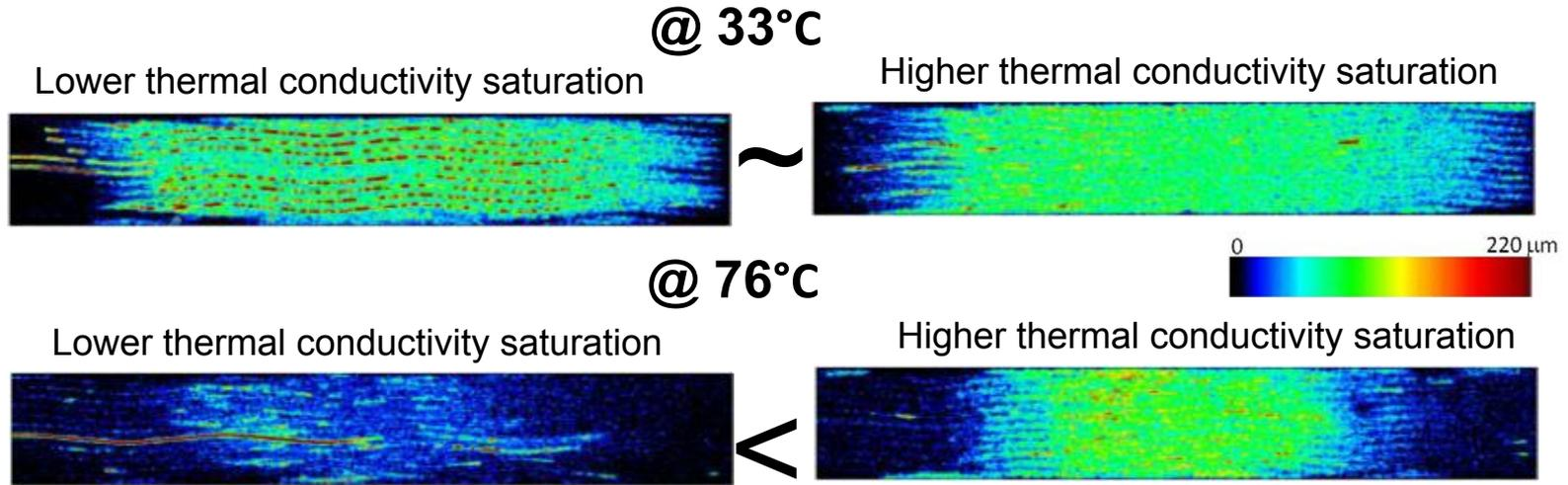
❑ The driving force for vapor transport is 10X higher at 76°C as compared to 33°C.
