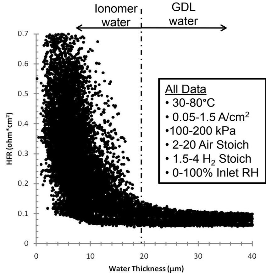
□ Liquid water required in GDL to minimize HFR as transition is very sensitive.
