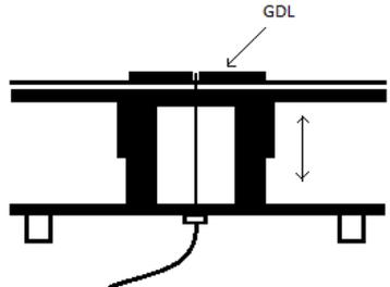
Injection of water drop through GDL for dynamic contact angle measurements.
