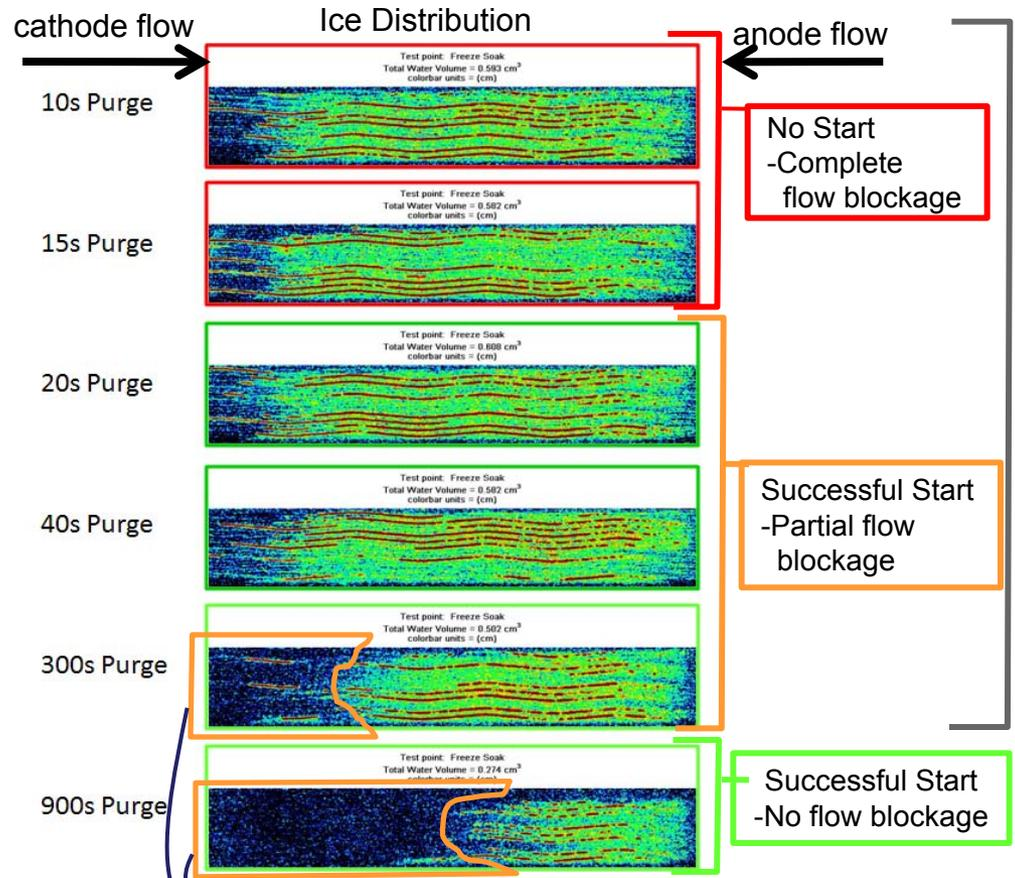
Evaporating water from porous layers extends run time while frozen, by providing space for additional ice formation and accumulation
