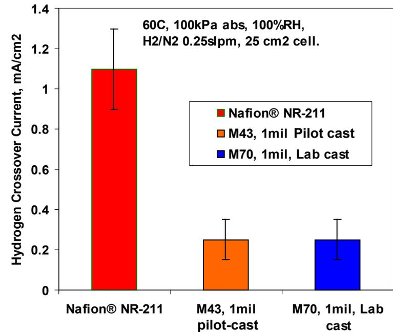
~75% less H<sub>2</sub> cross-over vs. Nafion® at equivalent thickness
