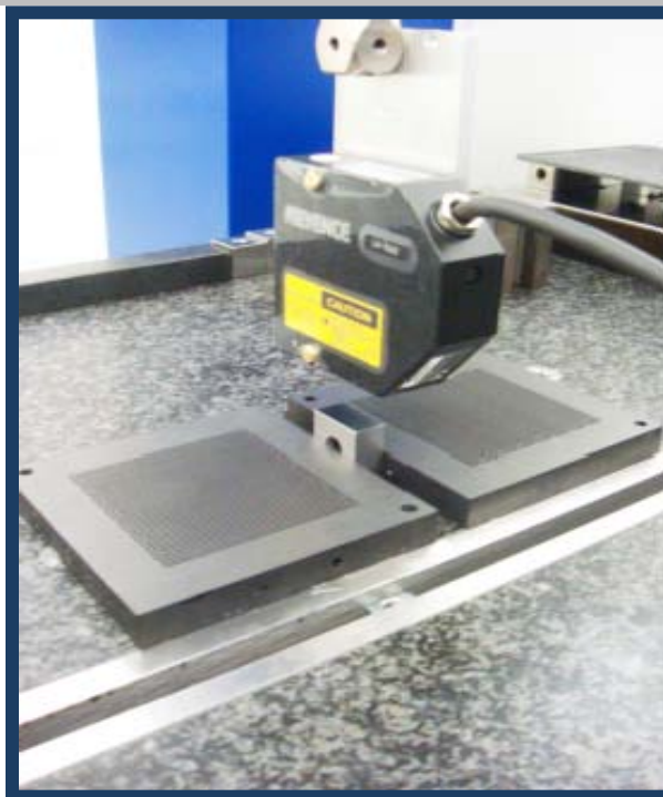
Non-Contact Sensor for Bi-Polar Plate Manufacturing Process Control and Smart Assembly - NIST
