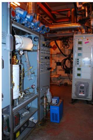
**High pressure screening: quantify durability & poison resistance**
