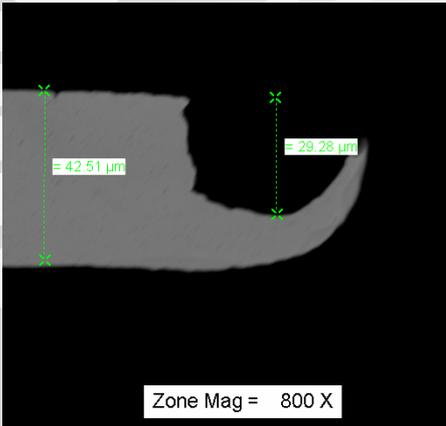
Cross-section of membrane failure point
