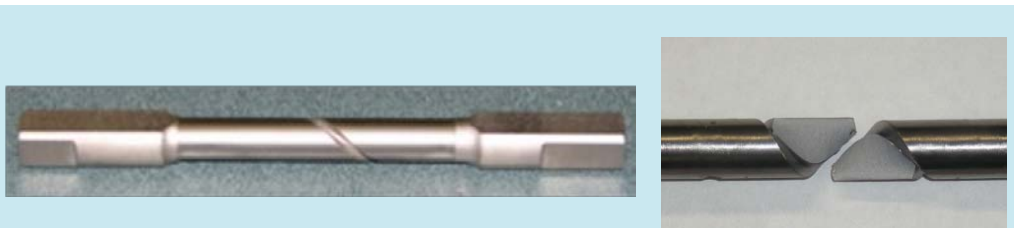
SNTT test specimen and fracture surface
