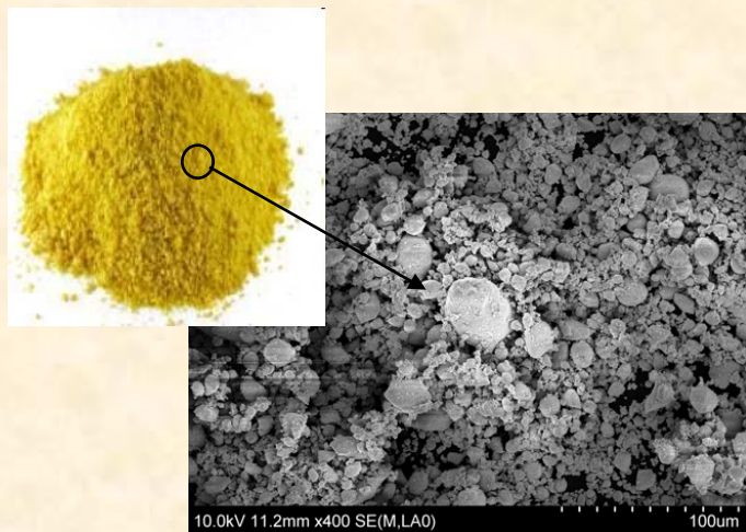
SEM micrograph of WO 3 nano-powder
