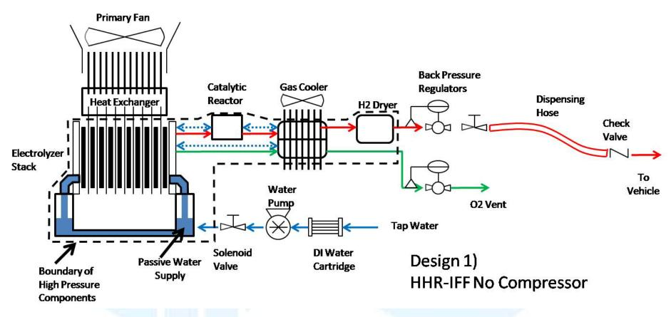
Schematic diagram showing the important mechanical system components, excluding sensors and electrical controls for the high pressure HHR-IFF electrolyzer system. Note that as much detail as possible is given to ancillary components, since they all contribute to cost.
