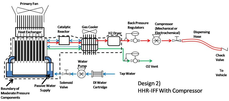
Schematic diagram showing the important mechanical system components, excluding sensors and electrical controls for the moderate pressure HHR-IFF electrolyzer system with a compressor added to reach 5000 psi. Note that as much detail as possible is given to ancillary components, since they all contribute to cost.
