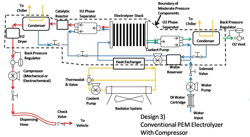
Schematic diagram showing the important mechanical system components, excluding sensors and electrical controls for the moderate pressure HHR conventional electrolyzer system with a compressor added to reach 5000 psi. Note that as much detail as possible is given to ancillary components, since they all contribute to cost.
