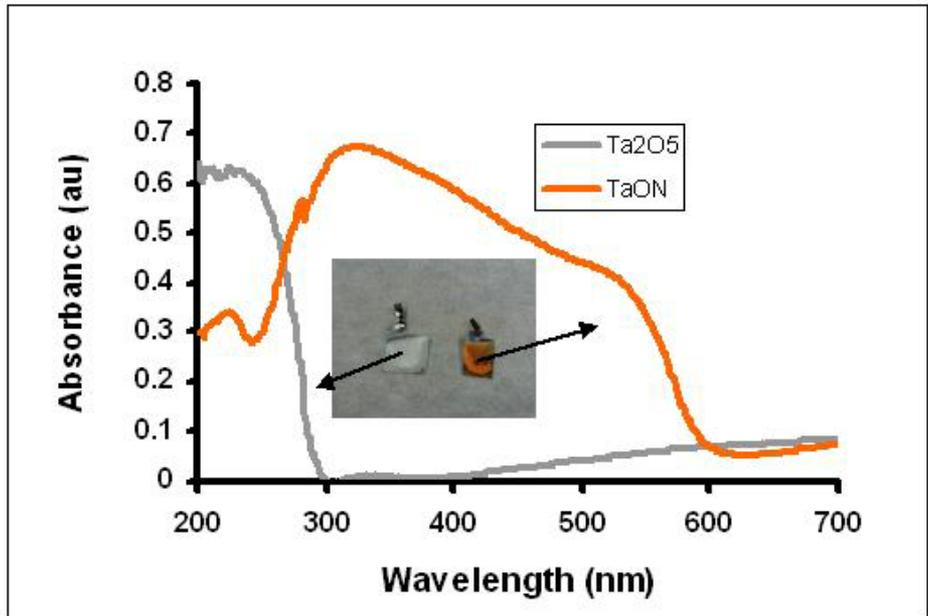
Fig. DRUV-Vis spectra of Ta<sub>2</sub>O<sub>5</sub> and TaON NTs
