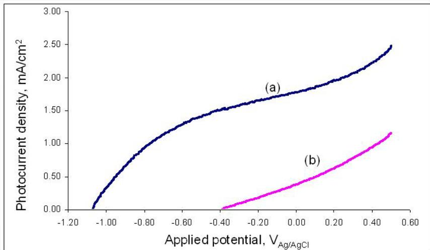
**Fig.** Potentiodynamic plot of TaON NTs under global AM 1.5 solar light (a) and visible light ( $\geq 420$  nm) illumination. Nanotubes of 50 nm internal diameter and 525 nm long are used. Sample area: 1 cm<sup>2</sup>
