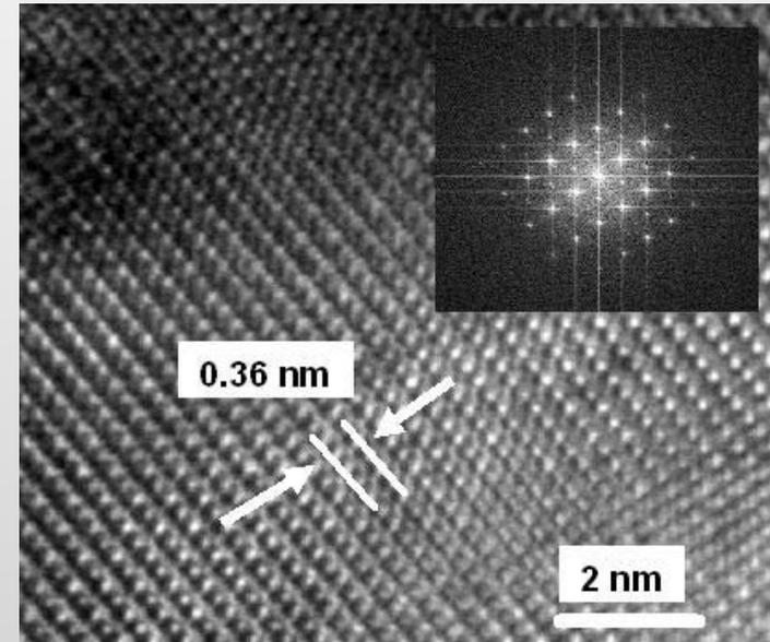
**Fig.** TEM image of TaON nanotube arrays
