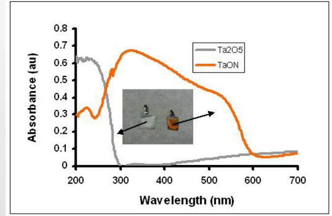
Experimental UV-Vis optical absorbance spectra of Ta<sub>2</sub>O<sub>5</sub> and TaON.
