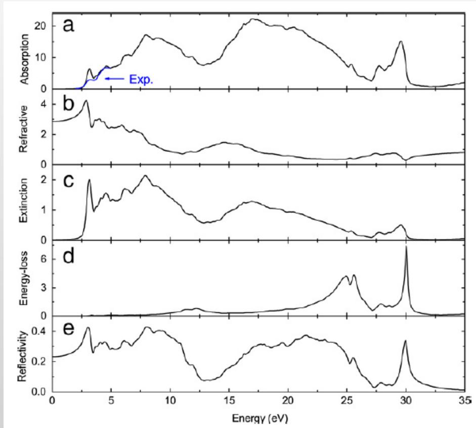
SP-GGA+U is used for calculation of the band structure and optical properties of BiFeO<sub>3</sub>, considering the unoccupied Fe 3d orbital state. The calculated band gap is 1.61 eV.
