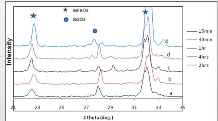
XRD patterns of BiFeO<sub>3</sub> annealed under N<sub>2</sub> at 600 °C for (a) 15 min, (b) 30 min, (c) 1 h, (d) 4 h and (e) 2 h
