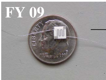
3 rd Gen ESL Prepared Sensor. Resistive heater Side Shown. Sensor weight about 1gram. Size: 3 mm Square
