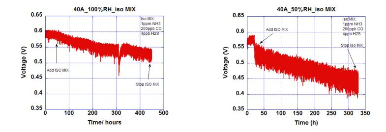
• Results shown reflect ISO mix with NH3, CO, and H2S at 100% RH and 50% RH, 80C, 30 psig
