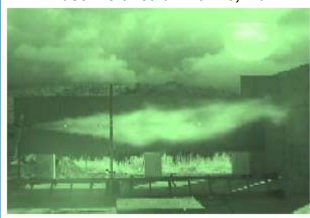
Horizontal Flame 3.6 - 4.3 m long, 0.6 - 1 m wide
